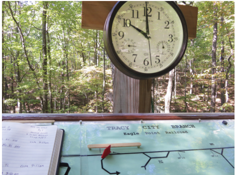
Figure 6: The Popsicle stick on the board is a reminder to the dispatcher to protect the extra train.
